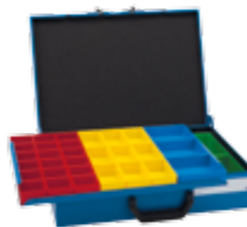
SMALL COMPONENTS CASE 332 E 1/1 KM 332 E 1/1 Ref. No. 1000001531 Dimensions (LxWxH): 440 x 330 x 100 mm Weight: 4.7 kg Inset boxes equipped lower: 12 x A3 red, 6 x B3 yellow, 3 x C3 blue, 2 x D3 green Inset boxes equipped upper: BES 31 1/1, 18 x A4 red, 9 x B4 yellow, 3 x C4 blue
